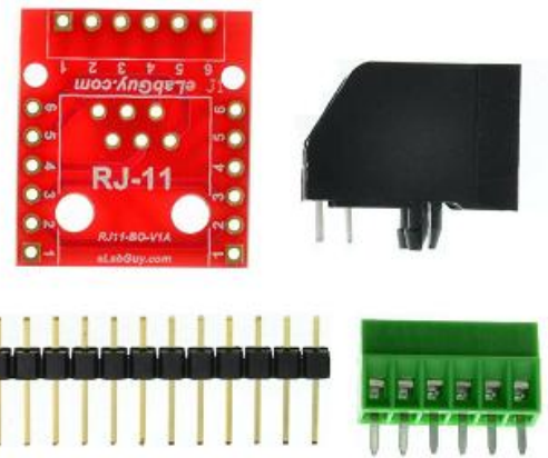
Figure 1: Parts inside the kit (Note: the module is not assembled, user can decide which connector to use on the module.)
