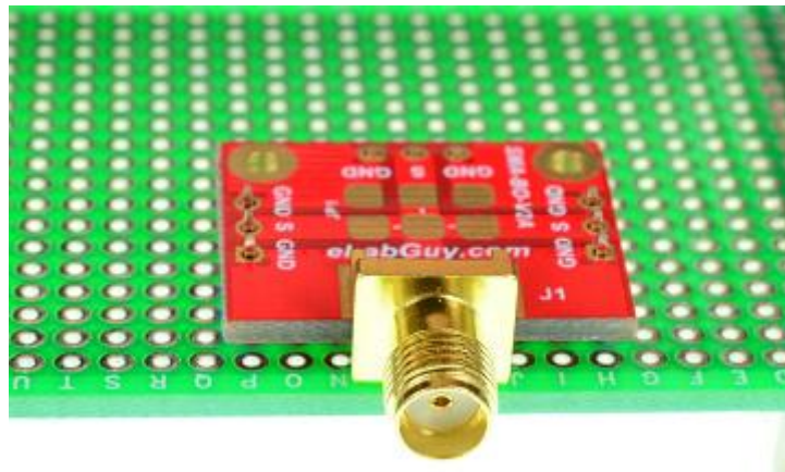
Figure 4: Solid Mounting on prototype PCB
