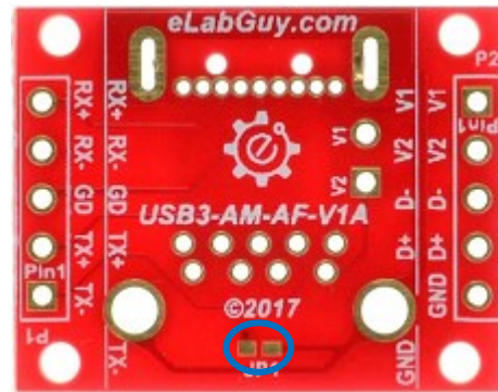
Figure 6: PCB back with optional Jumper connects Shield to GND
