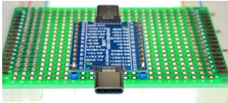
Figure 5: Solid Mounting on prototype PCB (Note: This picture only shows the pins spacing, actual use may not be used on a breadboard)
